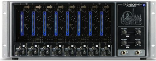
500ADAT is an 8-in/8-out ADAT expander that combines a 500 series rack with high-performance AD/DA conversion and ADAT I/O that allows any engineer to integrate the 500 series format into their studio using free ADAT I/O on the back of many popular audio interfaces.
