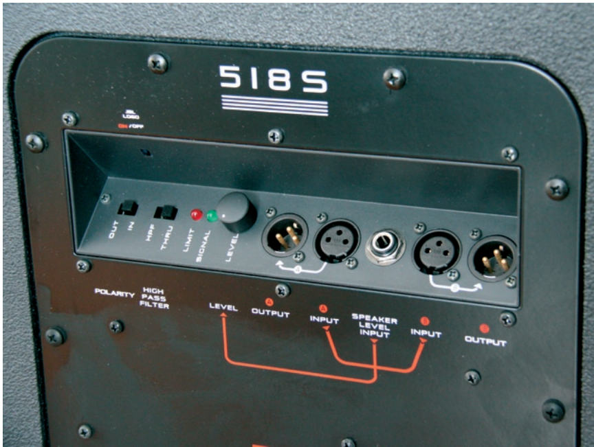
▲ The control panel on the rear of the 518S is equipped with two balanced XLR inputs and associated link outputs, a Speaker Level Input and control, High Pass Filter switch with full pass-through or high-pass options, and a Polarity switch.
